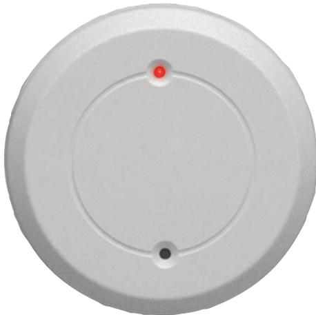
The DS1100i Detector Series uses microprocessor-based sound analysis technology (SAT) to listen for the specific frequencies associated with breaking glass. The DS1101i, DS1101i-BEL, DS1101i-CHI, and DS1101i-FRA can be used to detect breakage of plate, tempered, laminated and wired glass types. A built-in environmental test feature alerts the installer to false alarm hazards in harsh environments. The round detectors mount on the ceiling or walls.
