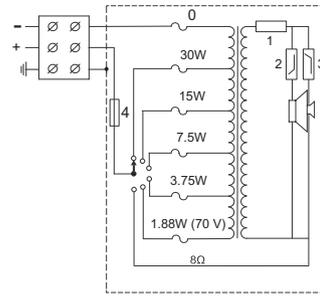
Circuit diagram (1: Passive Limiter, 2: Low Pass Filter, 3: High Pass Filter, 4: Thermal fuse)
