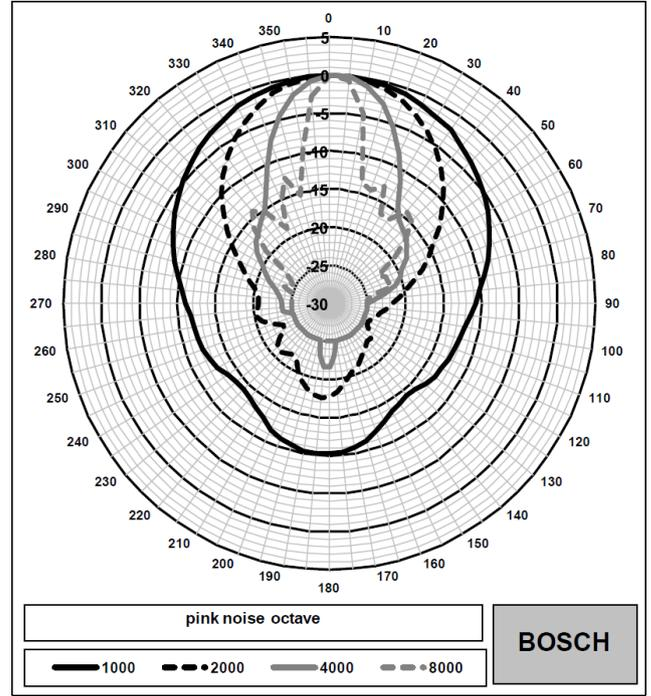
Fig. 7: Vertical polar diagram (high frequency part)
