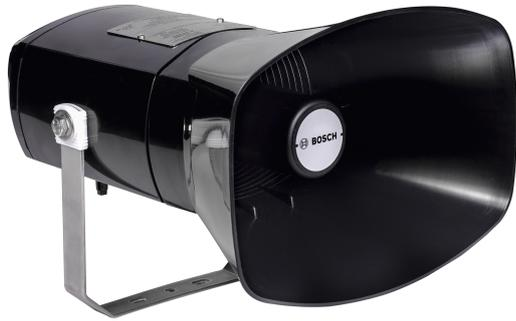
The LH3-UC25XL horn loudspeaker is specifically designed and certified for installations where explosive gas-air mixtures are likely to be present. The horn is constructed from anti-static Polyamid material, making the horn sturdy and light weighted. The longer flare design of the horn results in a higher sound pressure level where longer distance areas can be covered.
