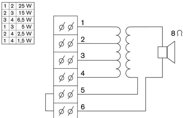
Fig. 2: Circuit diagram
