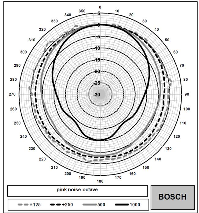
Fig. 6: Vertical polar diagram (low frequency part)
