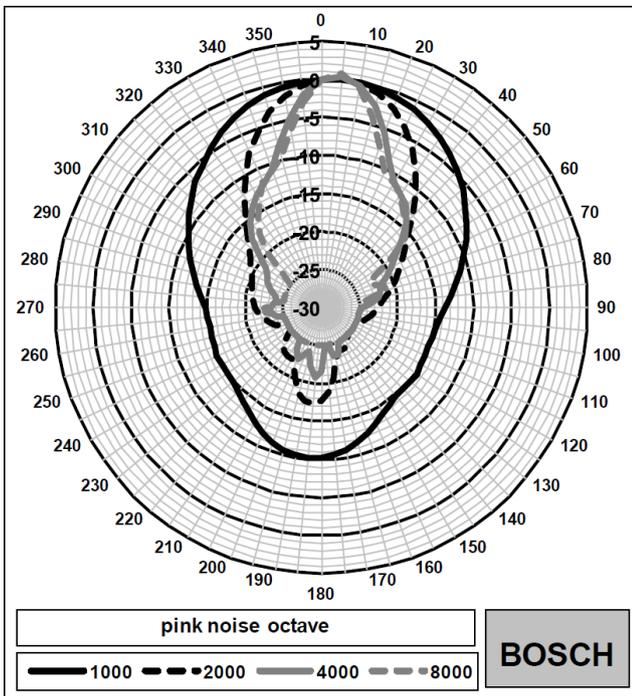
Fig. 5: Horizontal polar diagram (high frequency part)
