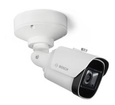
The NBE-3702-AL is a versatile device for general outdoor surveillance monitoring. The compact design for discreet use with quick set-up offers high installation flexibility. The camera offers a 1/2.8" sensor and HDR technology at HD 1080p. Combined with an integrated varifocal lens, the camera provides a sharp and detailed image with flexible field of view. With added IR functionality, the camera is able to function even in scenes where ambient lighting is not always available.
